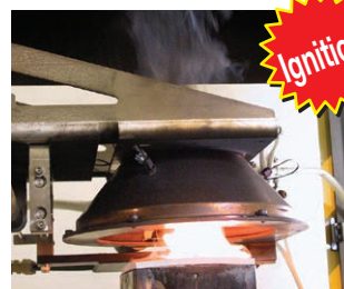
Test material size: 100 mm x 100 mm x 5 mm (thickness), measured at a radiation heat level of 50 kw/m 2
