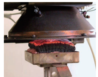
The material carbonizes without igniting.
