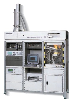
Test material size: 100 mm x 100 mm x 5 mm (thickness), measured at a radiation heat level of 50 kw/m 2
