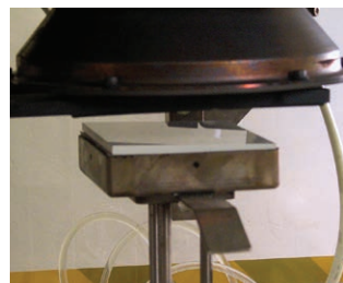
Fire ignited by a 10,000-V electric spark.
