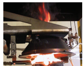
Test material size: 100 mm x 100 mm x 5 mm (thickness), measured at a radiation heat level of 50 kw/m 2
