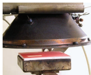
Test material size: 100 mm x 100 mm x 5 mm (thickness), measured at a radiation heat level of 50 kw/m 2
